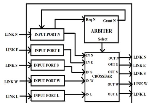
Figure 1. 5 x 5 Router architecture
