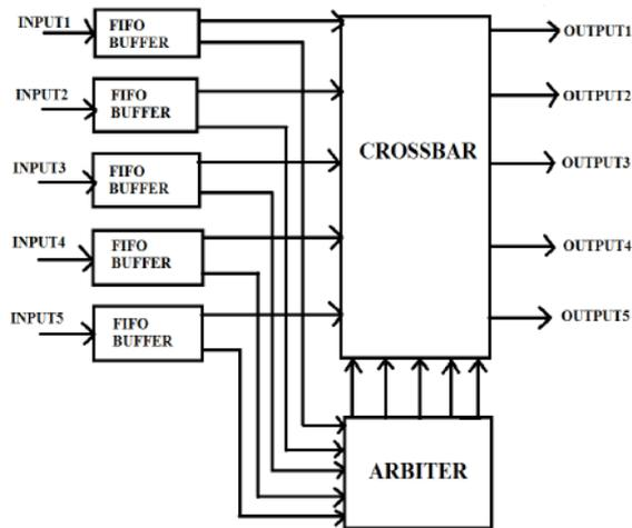
Figure 2. Schematic diagram of 5x5 Router architecture
