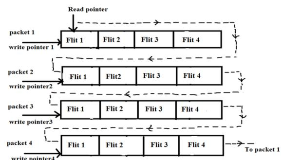
Figure 5. Read and write operations in FIFO
