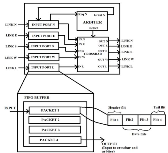
Figure 3. 5x5 Router architecture using buffering method
