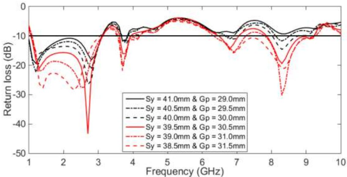
Figure 5: Return loss versus frequency plot of proposed antenna with variation ‘Gp’ and ‘Sy’ parameters
