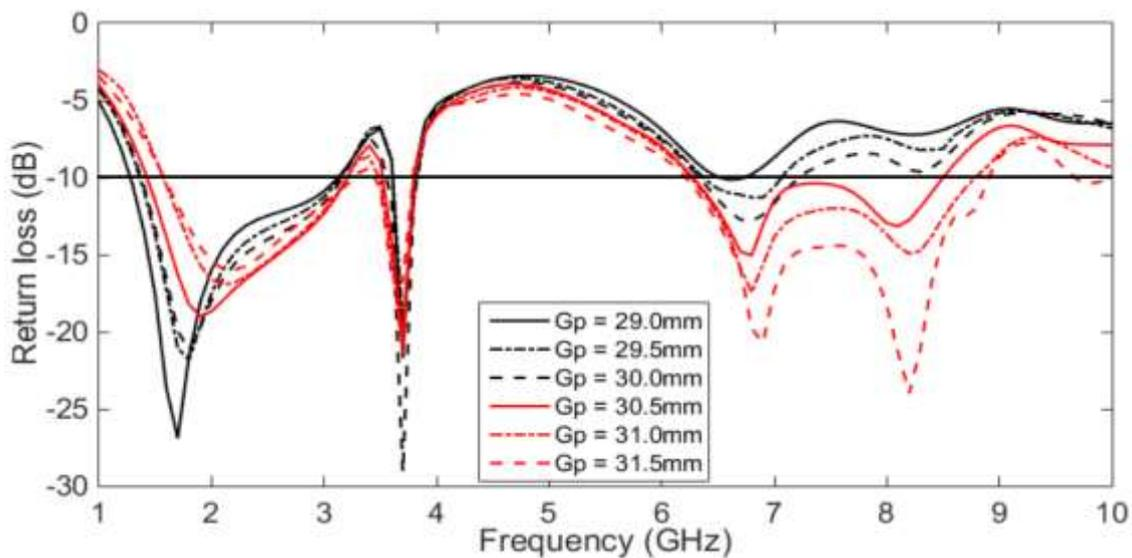
Figure 4: Return loss versus frequency plot of proposed antenna with ground length variation ‘Gp’
