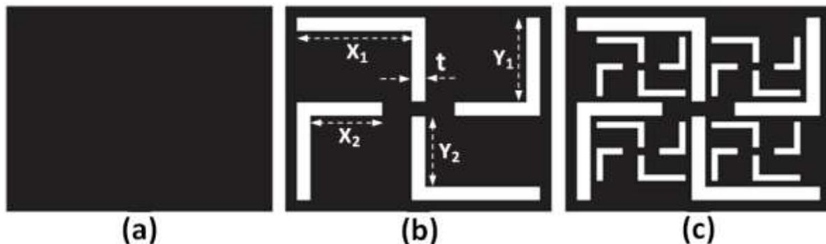
Figure 1: Design evolution for the patch of proposed antenna; (a) 0<sup>th</sup> iteration, (b) 1<sup>st</sup> iteration and (c) 2<sup>nd</sup> iteration (final patch geometry of proposed antenna)
