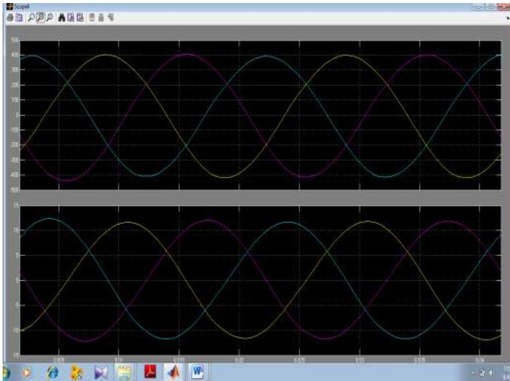
During the breaker in open condition the grid voltage will be maximum.(405 V)
