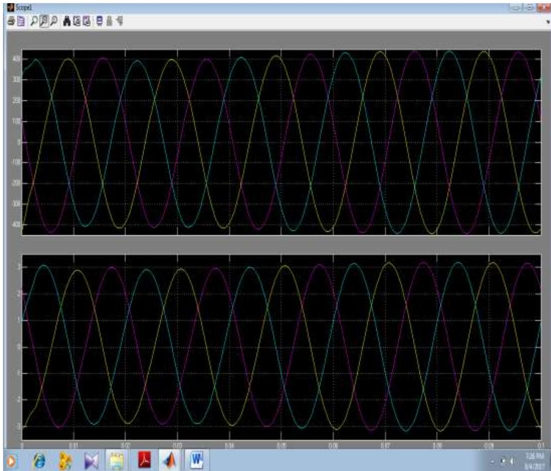
During the breaker closed condition the load take the voltage of 405 Volts
