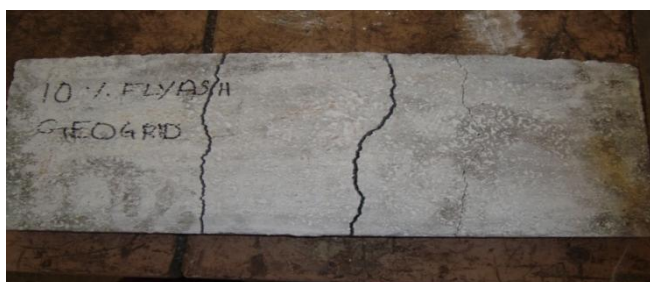
Figure 4.6 Failure of Geogrid mesh panel
