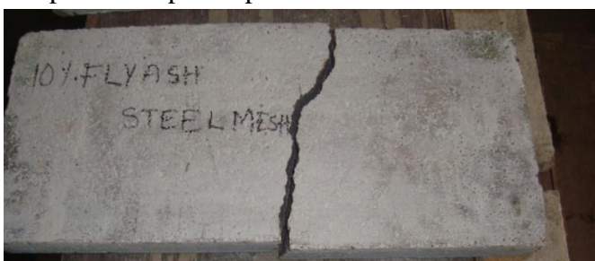
Figure 4.5 Failure of steel wire mesh panel
