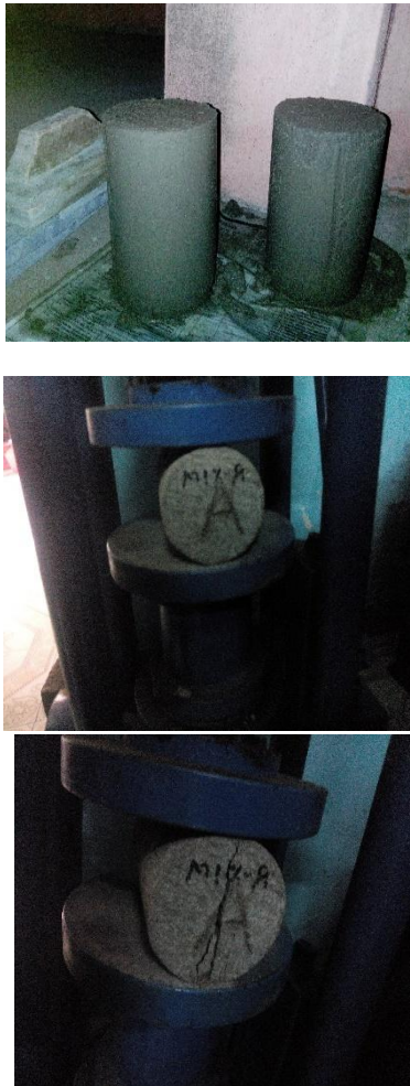
Figure 3.11 Casting and testing of cylinder
